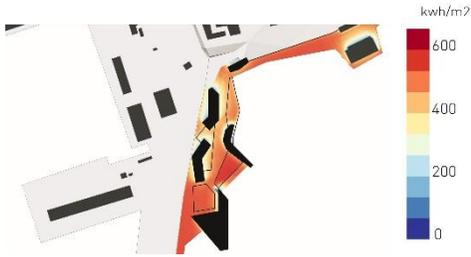
In the summer period almost all areas still fully exposed. As local mitigations, operable sun shading systems are proposed to lower the solar exposure.
