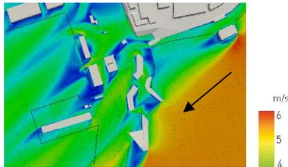
Analyzing the summer wind, the air distribution on the new layout is good. The new shape and orientation of the massing is allowing the South wind to flow through the areas without creating discomfort.
