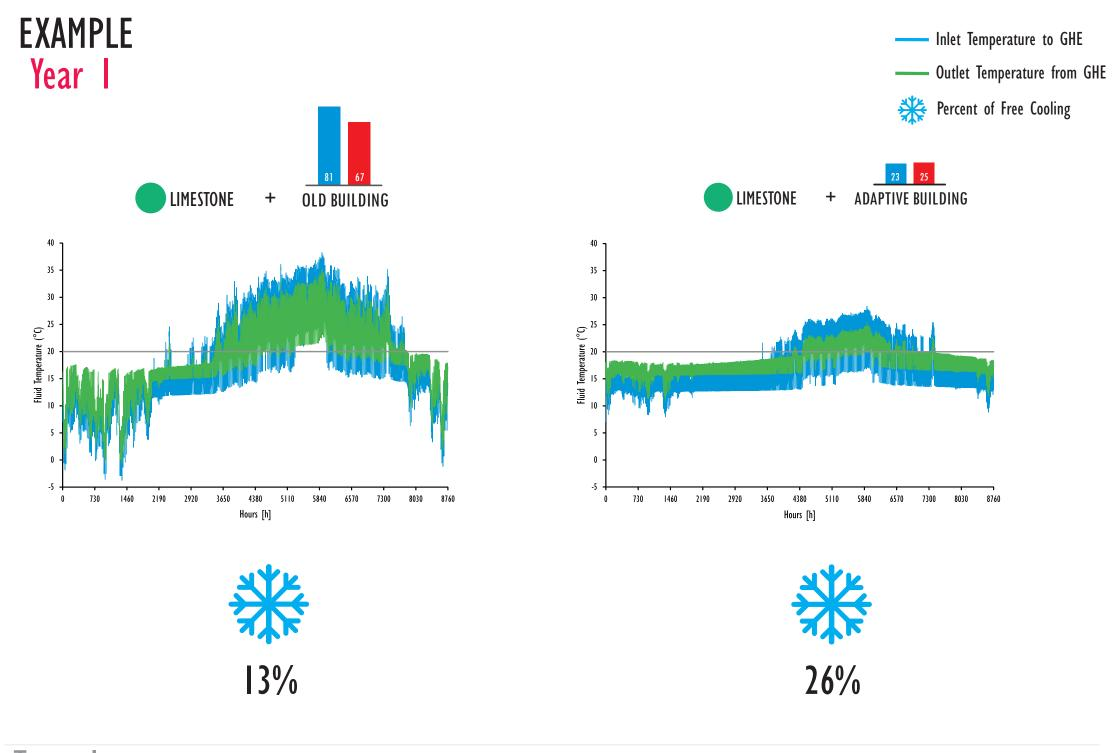
The graphs show the inlet and outlet temperatures of the heat carrying fluid in the ground heat exchangers (GHE) for the 1St year of operation.
