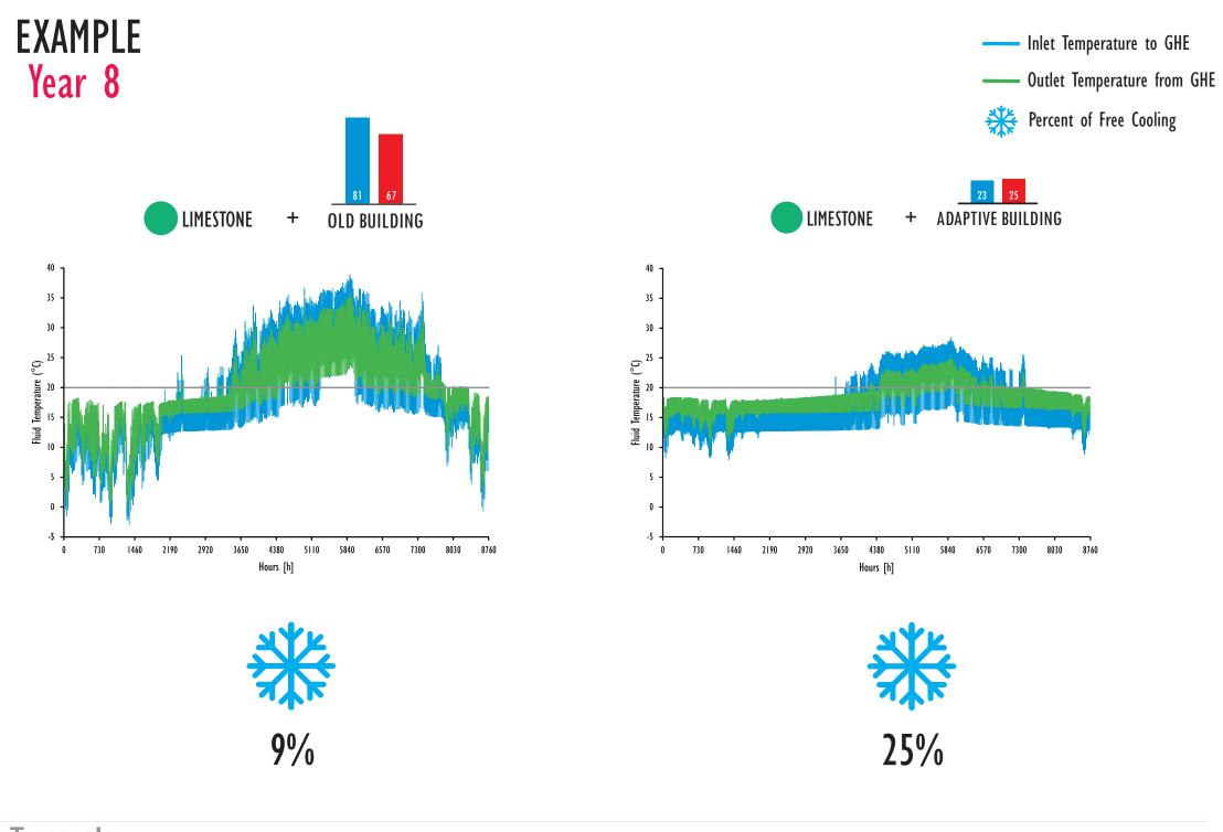
lhese graphs and numbers are for the 8th year of operation. Shifting between the two years clearly shows the effect of 'the unbalanced heating and cooling loads of the Old building. The ground gradually becomes warmer since the cooling demand is greater which means that more heat is being introducted than extracted from the ground. This is most obvious from the reduction in free cooling potential.
