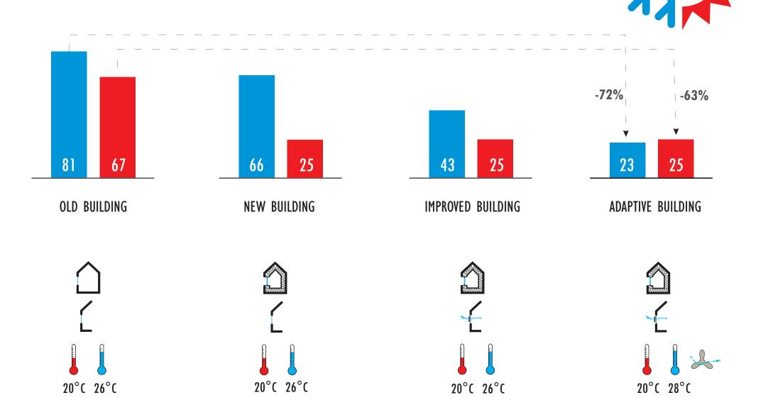
Shifting from the old building to the adaptive building reduces 72% of the cooling energy and 63% of the heating energy.
