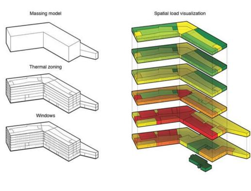
Once we have the unique Archetype Units, the next step is to create accurate representative energy models. This step is knøwn as Characterization.
