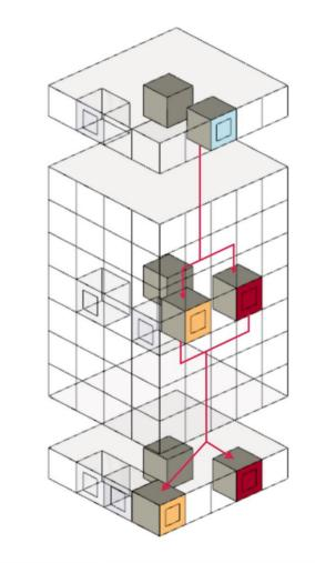
The first boundary condition assumption is that the surface temperature of the ceiling of a sheebox zone is at the same temperature as the average of the surface temperatures of floor of the sheebox zones above it (on the same facade orientation). In the case of zones on the top floor, the ceiling is treated as an external surface exposed to radiation.
