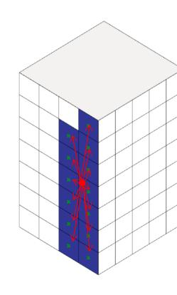
Once we have identified the different micro climatic (radiation) clusters, the next step is to place a representative sheebox energy model. If the similar radiation clusters occur at multiple locations on the facade, we find the centroid of the facade clusters, then identify the facade patch closest to the centroid.
