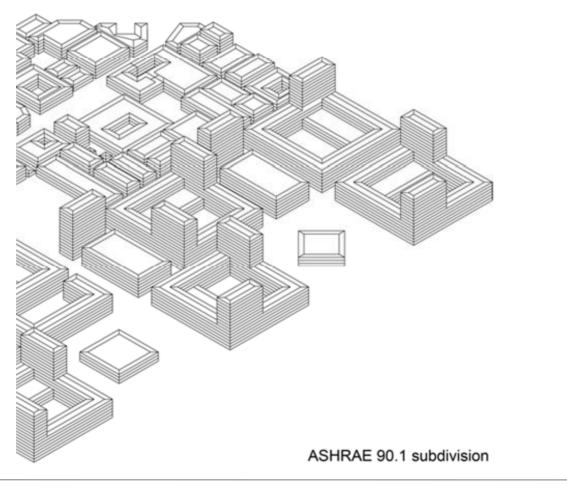
The most common rationalisation method is the division of the building geometry into Perimeter & Core Zones, as prescribed by ASHRAE 90.1 But this will still result in a very large number of simulation zones. Thus, further simplification is required.
