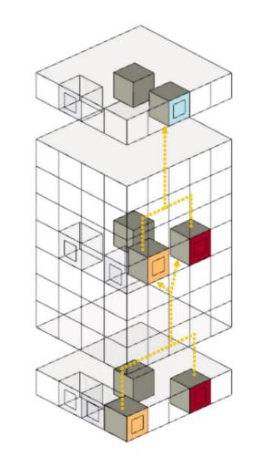
The second boundary condition assumption is that the surface of the floor of a shoebox zone is at the same temperature as the average of the surface temps of ceilings of the shoebox zones below it (on the same facade orientation). In case of ground floor zones, the floor surface temperature is treated the same as **Tsoil**.
