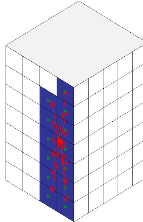
Once we have identified the different micro climatic (radiation) clusters, the next step is to place a representative shoebox energy model. If the similar radiation clusters occur at multiple locations on the facade, we find the centroid of the facade clusters, then identify the facade patch closest to the centroid.
