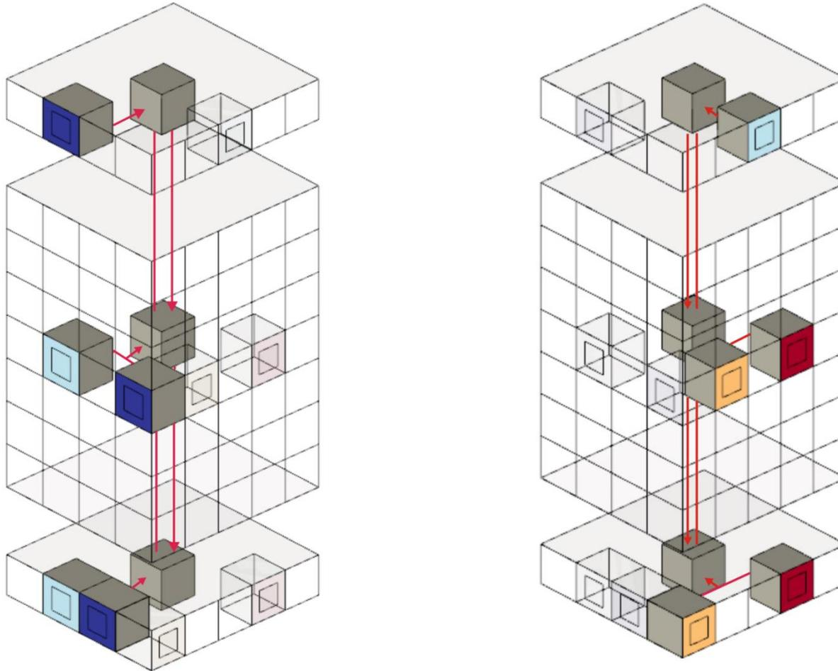
The fourth assumption is that the walls of a core shoebox are at the same temperature as back walls (that face the core) of a facade shoebox.
