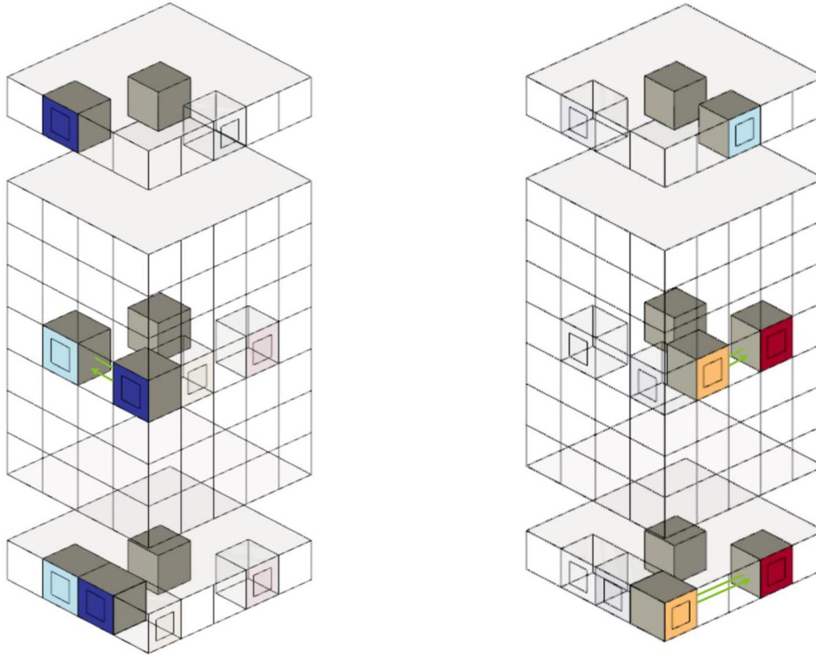
The third assumption about boundary conditions is that the side walls of a shoebox that face each other are at the same surface temperature
