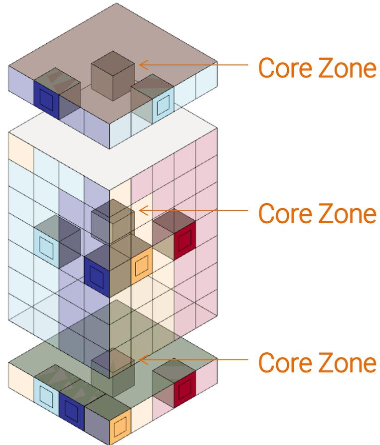
In addition to the facade or 'perimeter' shoebox zones, we place additional zones at the core, one each at the top, ground and middle floor.
