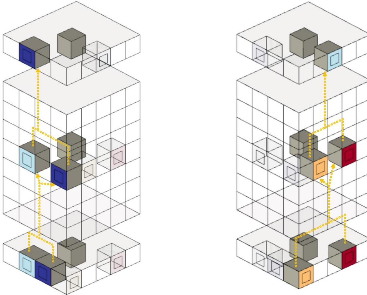
The second boundary condition assumption is that the surface of the floor of a shoebox zone is at the same temperature as the average of the surface temps of ceilings of the shoebox zones below it (on the same facade orientation). In case of ground floor zones, the floor surface temperature is treated the same as  $T_{soil}$ .
