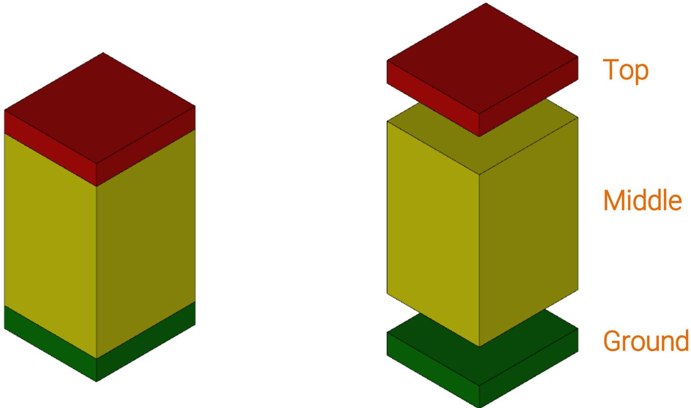
We begin by dividing each representative archetype unit into the **Roof**, **Ground** and **Intermediate Floors** to account for the different boundary conditions. (**Top floor roof + facades exposed to radiation ; Intermediate floors only facades exposed ; Ground floor facades exposed and heat exchange with the ground**)
