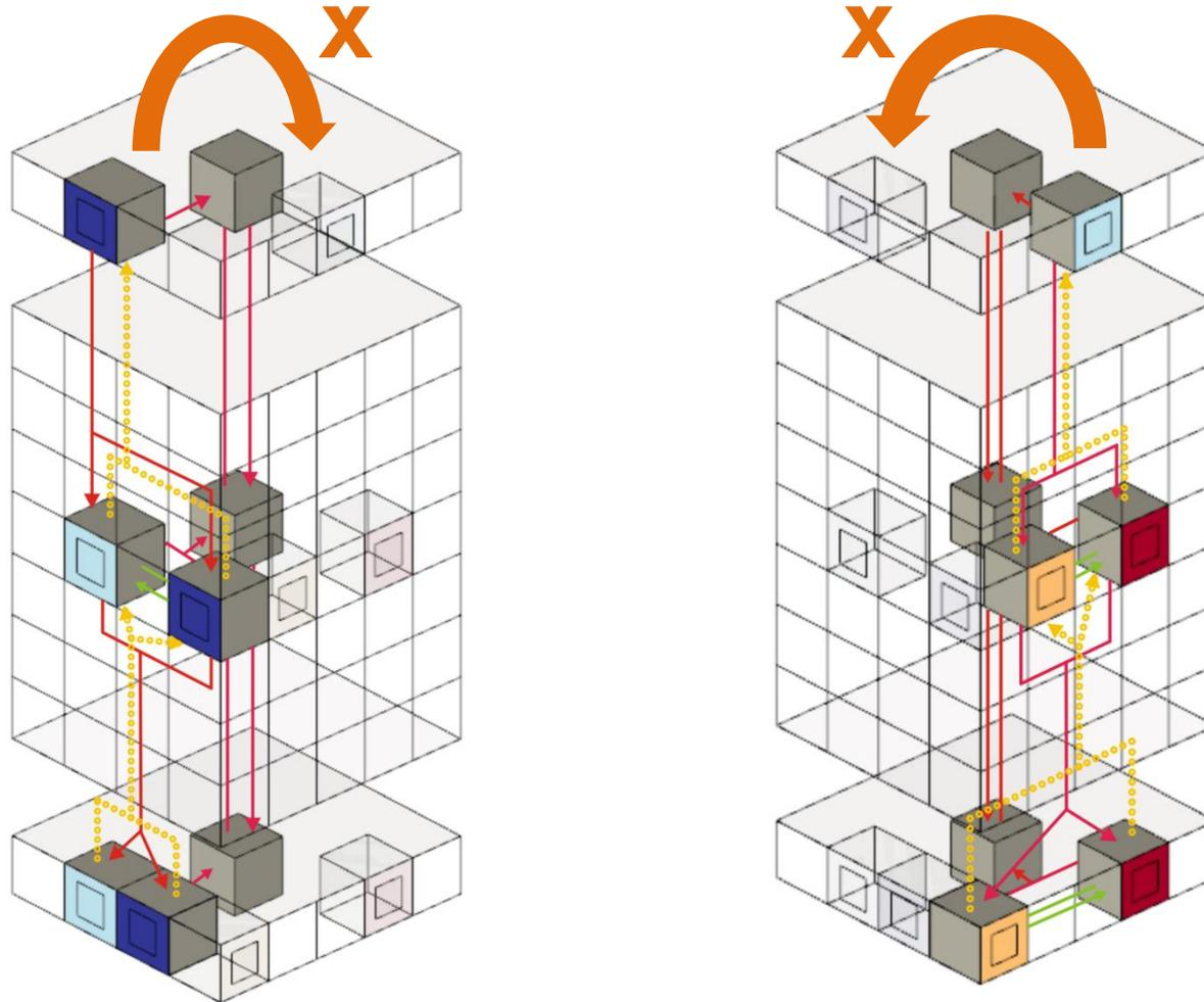
The sixth assumption is that the facade zones at one orientation do not exchange surface temperature information with facade zones at a different orientation. All temperature information exchange between facade zones at different orientations takes place through the core zones.
