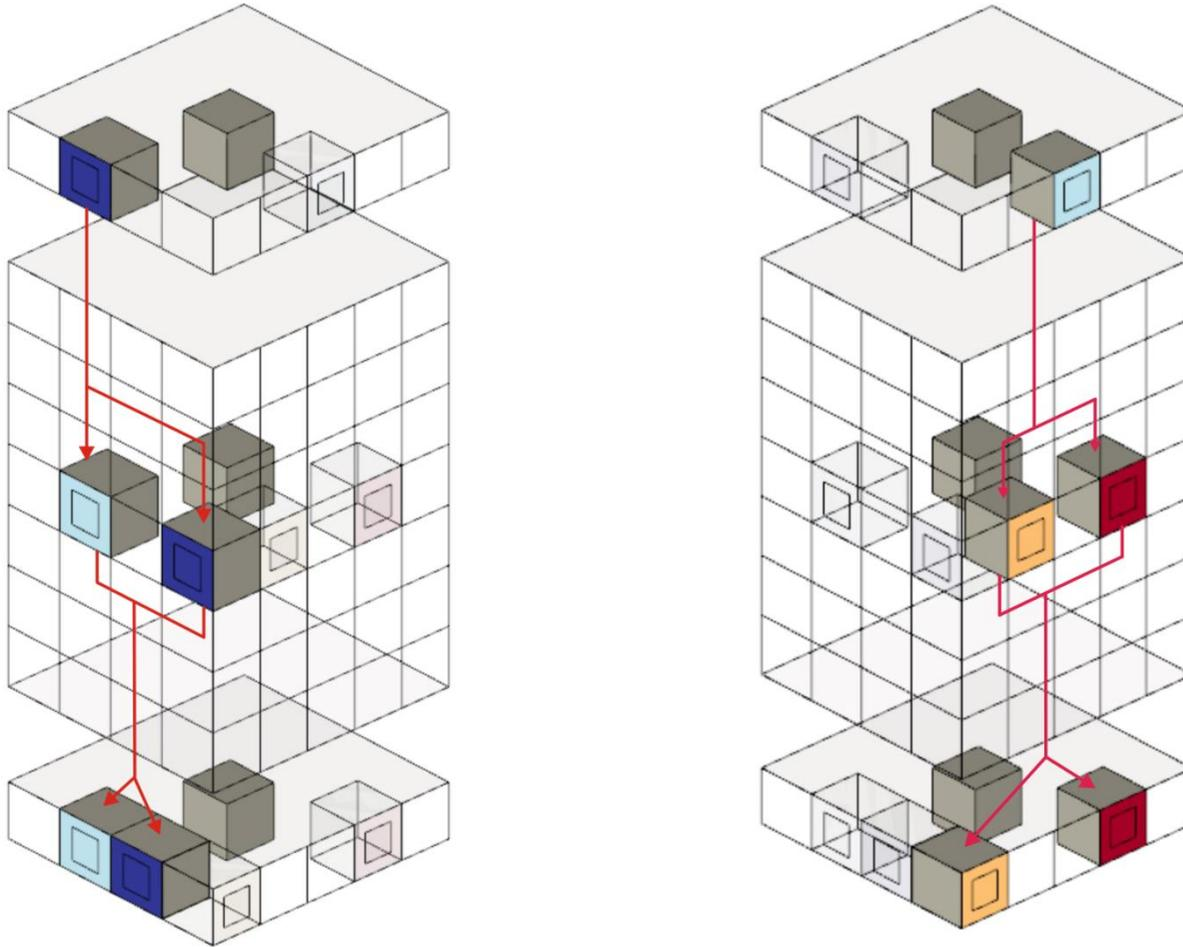
The first boundary condition assumption is that the surface temperature of the ceiling of a shoebox zone is at the same temperature as the average of the surface temperatures of floor of the shoebox zones above it (on the same facade orientation). In the case of zones on the top floor, the ceiling is treated as an external surface exposed to radiation.
