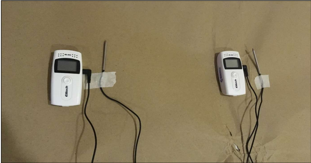
Figure 21 Incorrect placement for the Elitech devices external sensors
