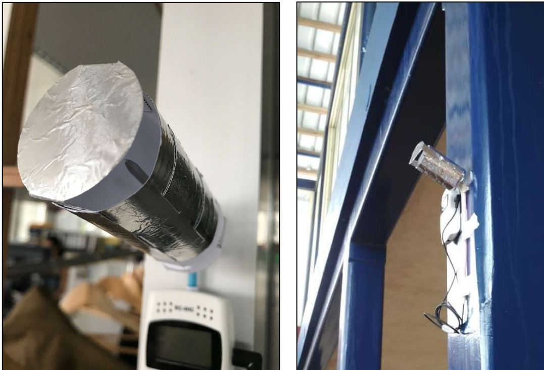
Figure 12-13 Prototype built by the author, notice the probe inside (left), and its application in the building
