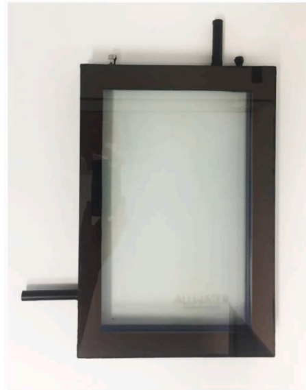
Appendix Fig. 1. Water-filled Glass prototype used for measurements [52].
