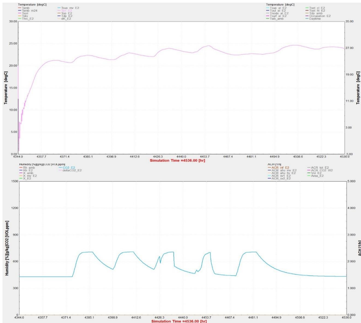
Figure 4.7 Screen capture of computer simulation model result of Kolbermoor, showing indoor air temperature and CO2 for 1st- 8th July 2018.
