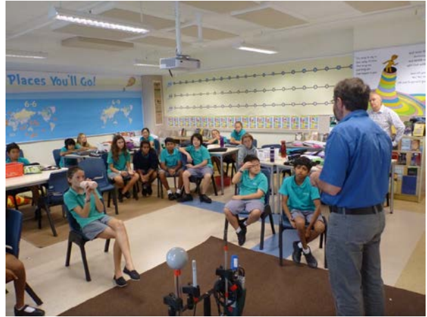
Figure 4: Testing of thermal comfort with elevated air speed at occupied class room in UWC, front: comfort sensors
